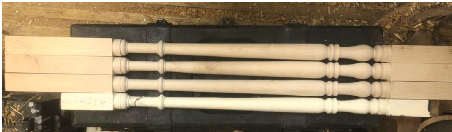
Stair Spindles in Sycamore
